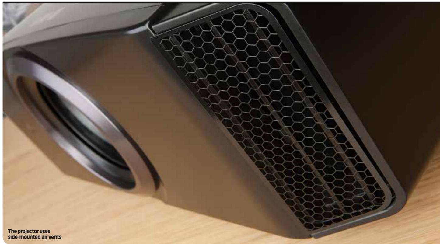
The projector uses side-mounted air vents
